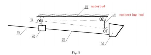
[21] It can be understood that the elastic rod 300 is not limited to being fixed to the underbed 100 and hinged to the water tank 220. It can also be fixed to the water tank 220 and hinged to the underbed 100. In this way, the purpose of stabilizing the pumping system 200, buffering vibration impacts, and reducing vibration transmission can also be achieved.
